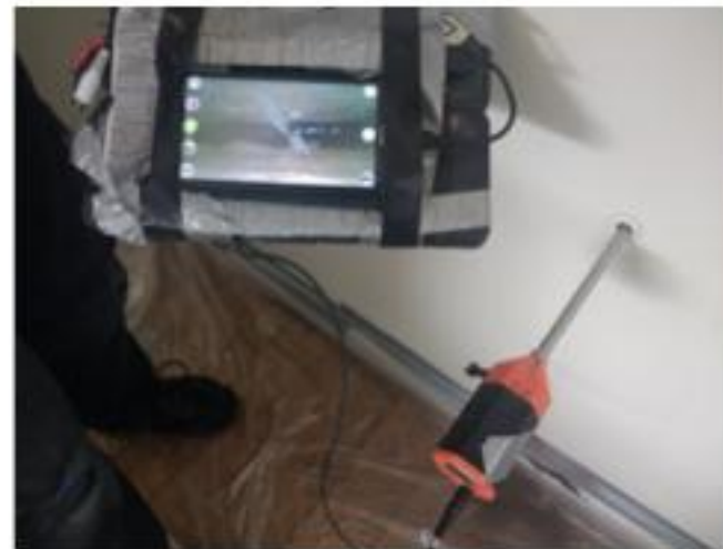
Boroscope surveys being undertaken to cavity brick/stone wall (above) Archive drawing: Precast concrete window surrounds (Right)
