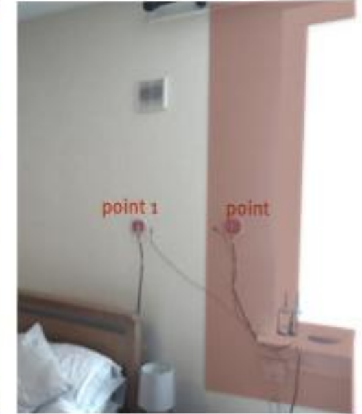
Existing in-situ U-value monitoring: Point 1 = 1.6 and 2 = 2.2W/m 2 K
