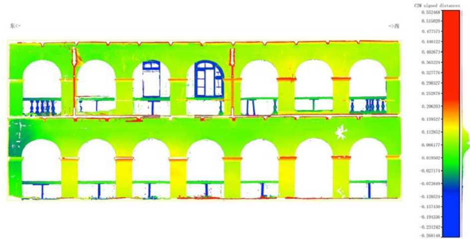
Analysis of the undulation of the south facade inside the building © CHCC
