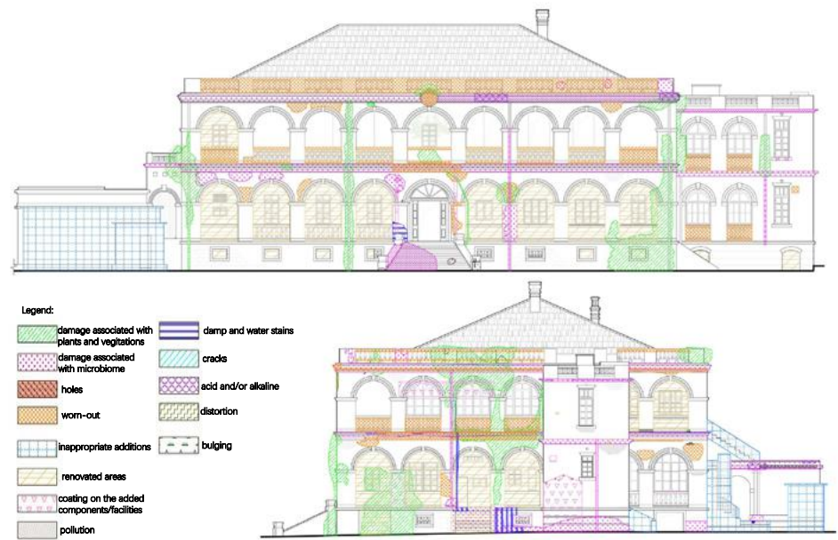
Analysis of the facade wall distress © CHCC
