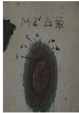
Analysis of door/window paint layers © Zhang Guangwei
