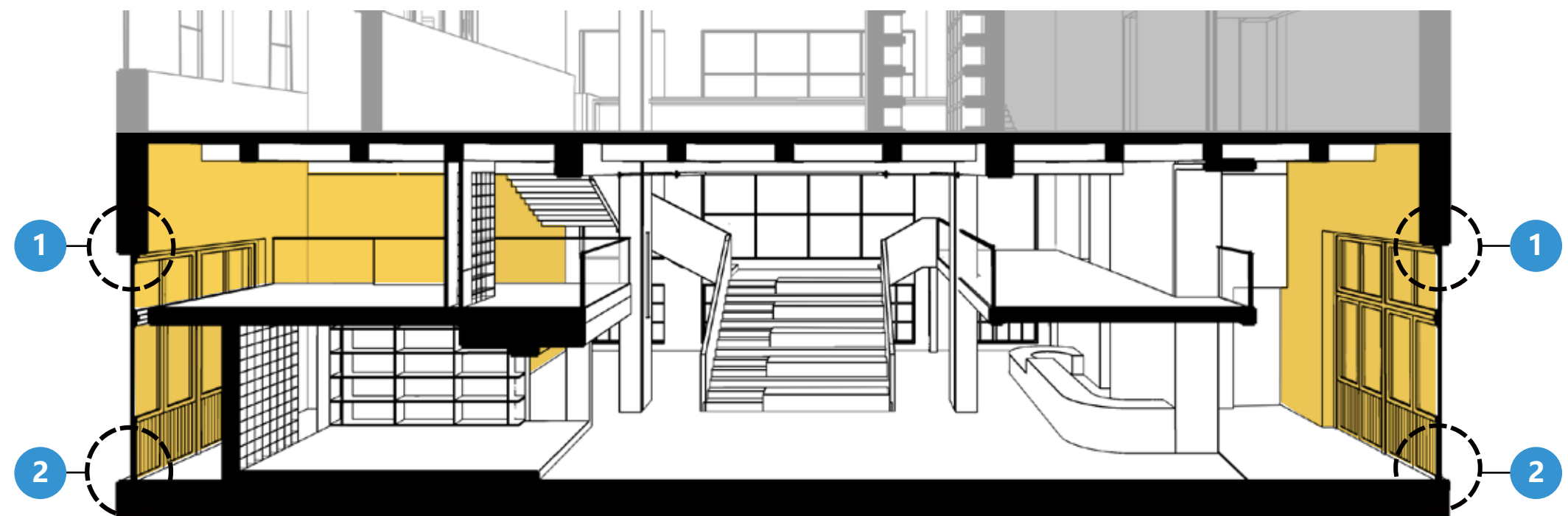
Newly built-up walls to improve insulation at entrances
